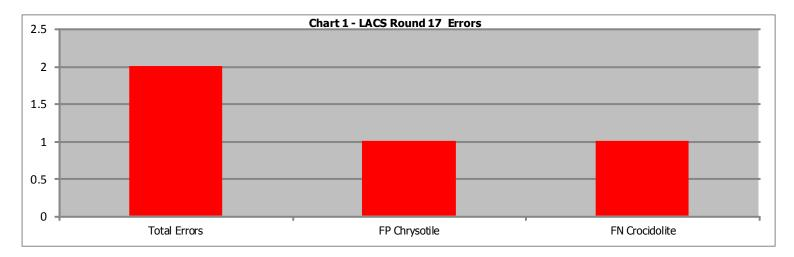
False Negative = Component has been missed. False Positive = Component has been incorrectly identified as present.
