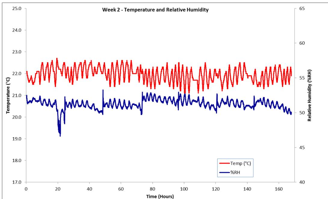
Figure 5: Temperature and Humidity Data – 168 to 336 hours of the 14 day test
