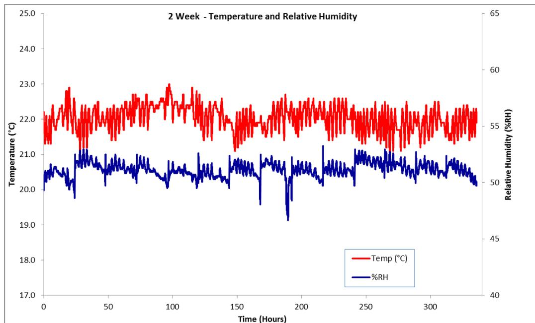
Figure 6: Temperature and Humidity Data – 0 to 336 hours of the 14 day test
