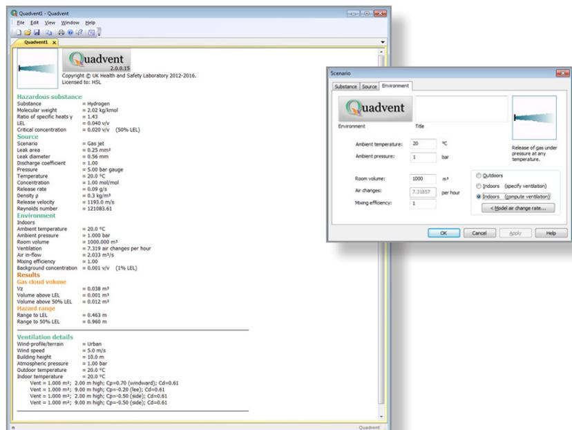
**Figure 3:** Calculation of the hazardous volume,  $V_z$ , using **Quadvent 2** for an indoor hydrogen release at 5 bar gauge. The inset window shows the dialogue box for changing the hole size for a releases under adverse conditions.
