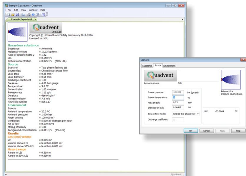
**Figure 1:** Calculation of the hazardous volume,  $V_z$ , from **Quadvent 2** for an indoor release of pressure liquefied ammonia. The inset window shows the dialogue box for inputting or adjusting the details of the source of the release
